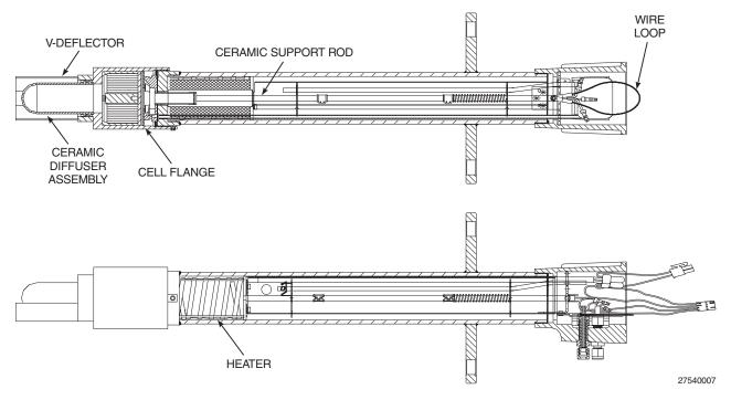
Figure 4-3. Heater Strut Assembly
